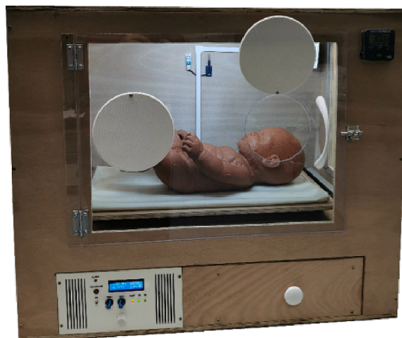
Fig. 2. Movable lids of the front window and the hinge-latch mechanism for its opening.
